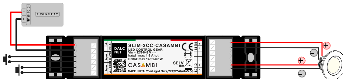
Figure 3: Wiring diagram for Tunable White / Dim to Warm LED loads
